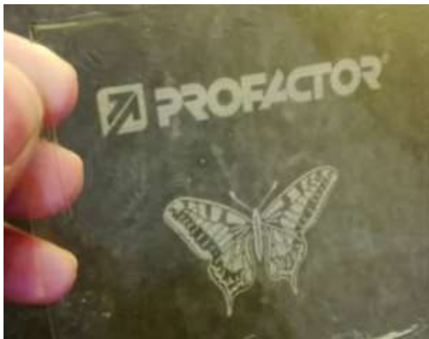
Figure 2: sample according to the layer stack in figure 1, but with inkjet deposited high refractive index material.
